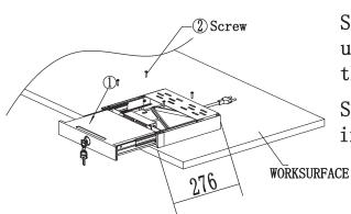
STEP ①: Put the power drawer box under the worksurafce and pull out the drawer
